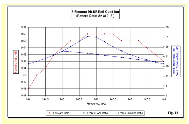
Beginning with the square quad properties over the 2-meter band, we may look at the gain and front-to-back curves in **Fig. 11**. Note that the gain and front-to-back peaks are well centered in the passband. The front-to-sidelobe ratio is a measure of the worst-case front-to-back ratio for the array. It will always be a curve that either overlays the 180-degree front-to-back curve or departs from it in a shallower curve at somewhat lower values.
