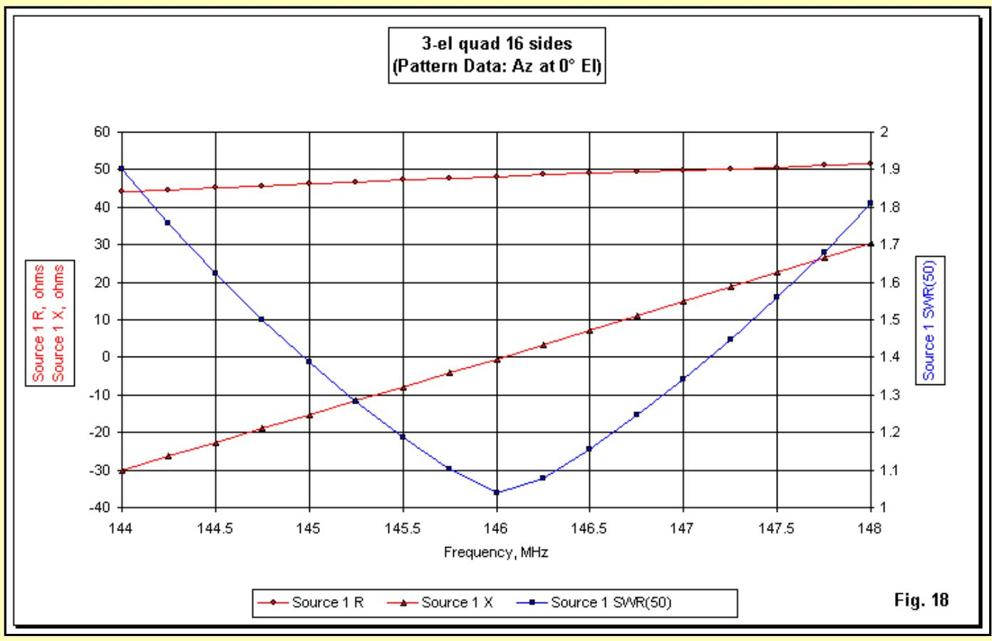
The bottom line, then, is that we may adjust a square quad to a circular loop quad by adjusting both the loop circumferences and element spacing. However, we should expect a slight reduction in the operating bandwidth. As well, the design might well use further optimizing to return the gain peak to the design frequency.
