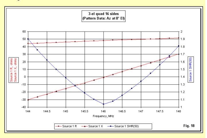
The bottom line, then, is that we may adjust a square quad to a circular loop quad by adjusting both the loop circumferences and element spacing. However, we should expect a slight reduction in the operating bandwidth. As well, the design might well use further optimizing to return the gain peak to the design frequency.
