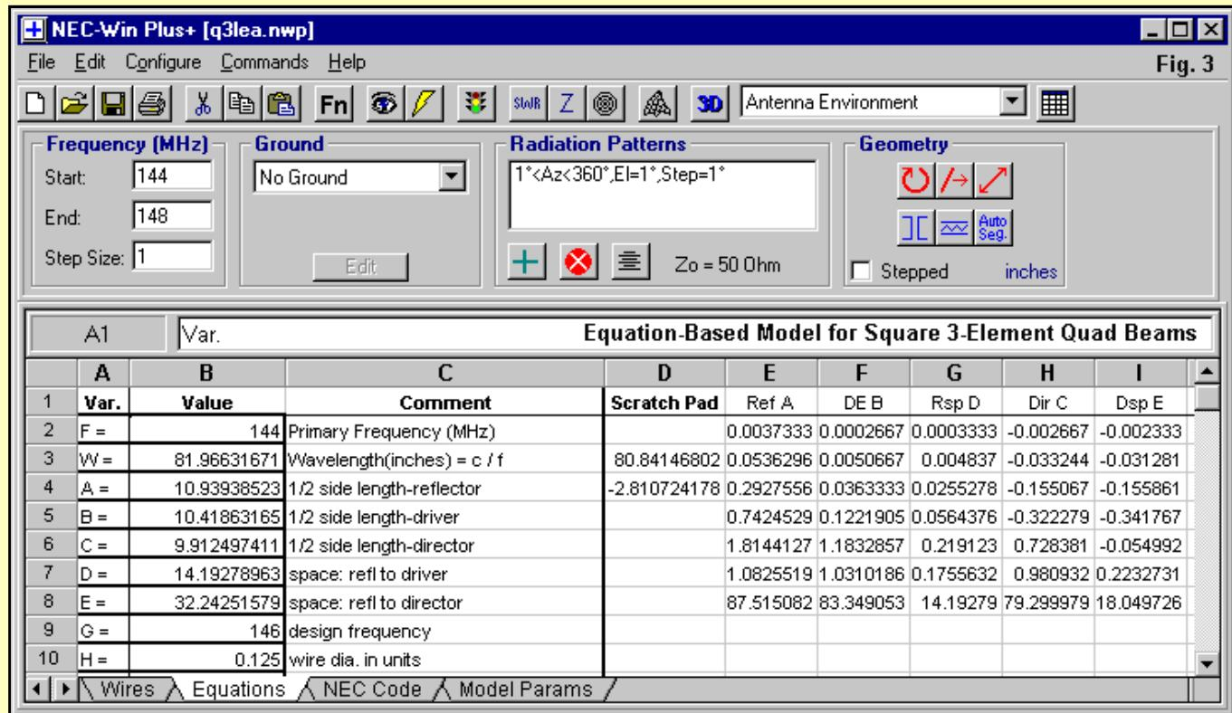
**Fig. 3** shows the equations screen for the model for a square 146-MHz quad using 0.125" diameter elements. This model requires only the revision of the variables for the wire diameter in the units of measure selected for the model and the design frequency (variables G and H). The remaining variables are calculated to yield half-side lengths and reflector to driver or director spacing for use in the model itself.
