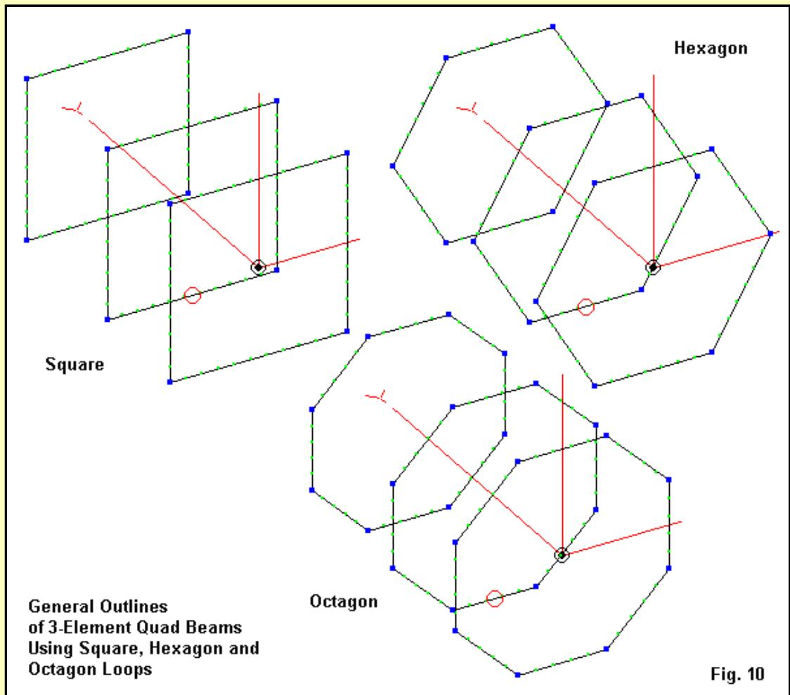
Although the main elements of comparison among the square, hexagon, and octagon arrays are easily observable from data tables, it may be useful to do a bit of graphic analysis on at least one array as a guide to interpreting the tables. For this sample run, I shall use 0.125" diameter wire and look at the square and the octagon versions of the quad after optimizing the octagon version for resonance at 146 MHz.
