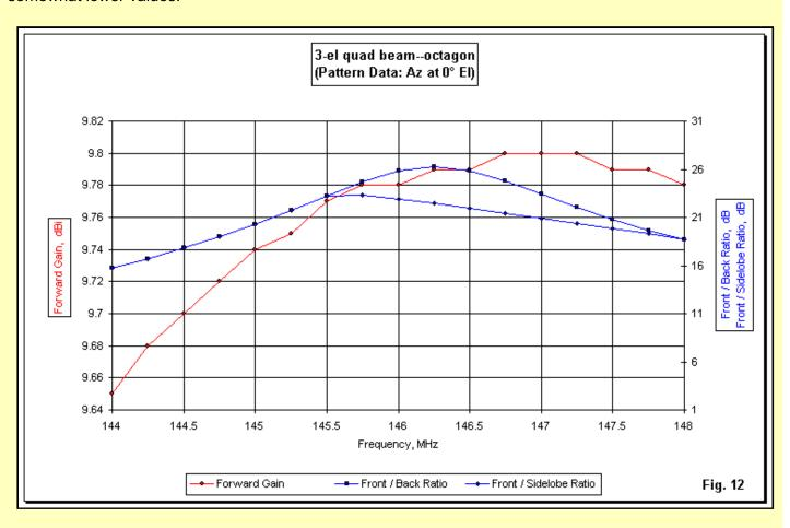
**Fig. 12** shows the comparable curve for the adjusted octagon array using the same wire size and element spacing. For the same resonant frequency, the octagon version shows a 180-degree front-to-back peak slightly above mid-band and a gain peak very much above mid-band. This pattern appears in all of the quasi-rounded versions of the arrays and indicates that changing shape has consequences for the performance curves.
