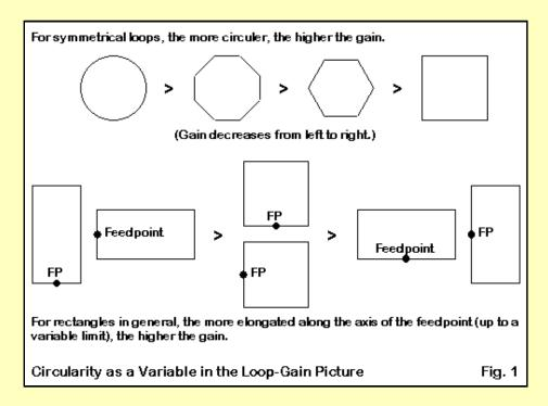
First, as portrayed in **Fig. 1**, the generalization is incomplete in its context. As shown in the top portion of the figure, it is more proper to say that among symmetrical loops, the circular shape has the highest gain of all of the possible polygon substitutes. The greater the departure from circularity, the lower the gain, if we maintain a regular polygon shape.
