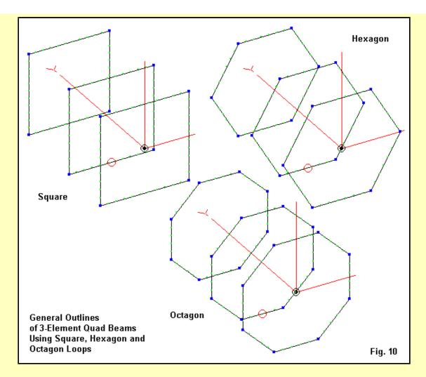
Although the main elements of comparison among the square, hexagon, and octagon arrays are easily observable from data tables, it may be useful to do a bit of graphic analysis on at least one array as a guide to interpreting the tables. For this sample run, I shall use 0.125" diameter wire and look at the square and the octagon versions of the quad after optimizing the octagon version for resonance at 146 MHz.
