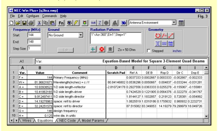
**Fig. 3** shows the equations screen for the model for a square 146-MHz quad using 0.125" diameter elements. This model requires only the revision of the variables for the wire diameter in the units of measure selected for the model and the design frequency (variables G and H). The remaining variables are calculated to yield half-side lengths and reflector to driver or director spacing for use in the model itself.
