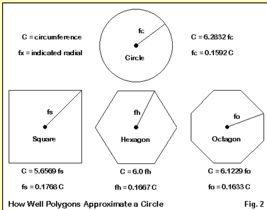
We know that the circumference of a circle is 2 times PI times the radius of the circle, and that the inverse lets us compute the radius from the circumference. The figure gives us the final numbers to 4 decimal places.
